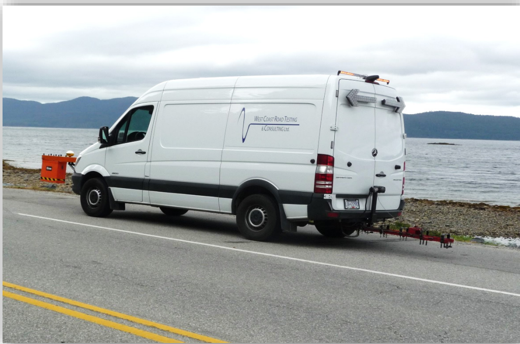
West Coast Road Testing FWD and GPR
