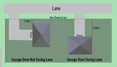
Garages with an overhead door facing a Lane must be setback a minimum of 3.0m
